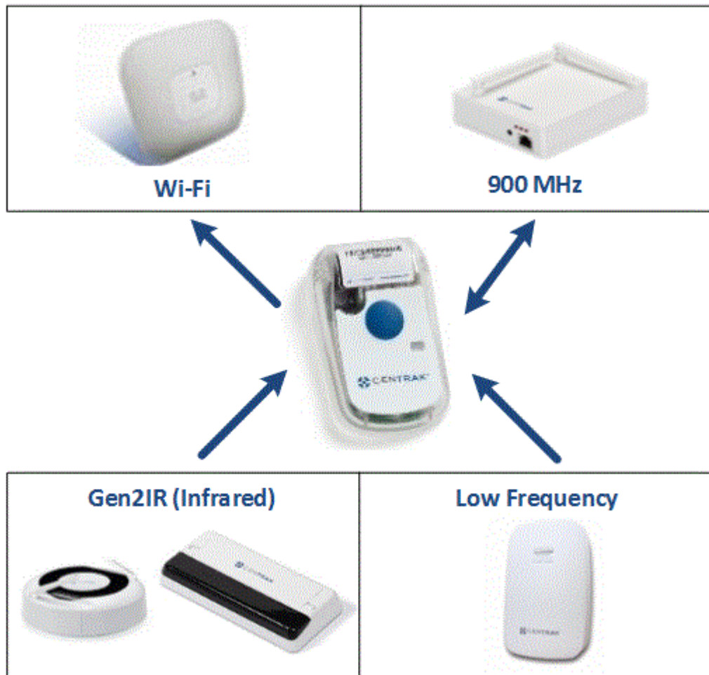
Figure 38: CenTrak Multi-Mode Tag – transmission and receiving capabilities
